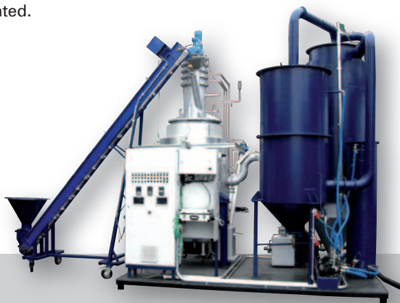
150 kW thermochemical converter (gasifier unit) after final installation and inspection. Conveyor belt (pellet feed charge), control unit, thermochemical converter (gasifier), gas cooling and cleaning (from left to right).
